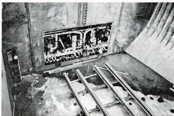
FIG. 5—Forward engine room bulkhead of Cape Horn showing a section removed prior to withdrawal of engines, and separate access door
