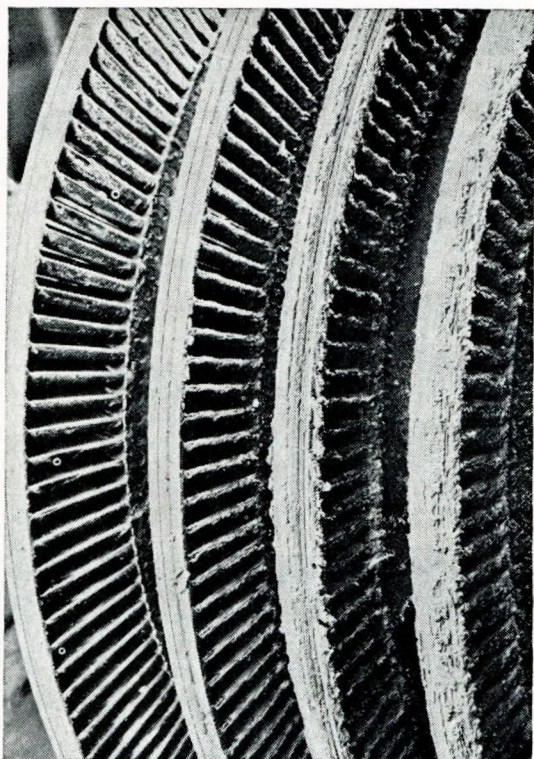
FIG. 12—s.s. Melania —fouling of HP turbine blades
