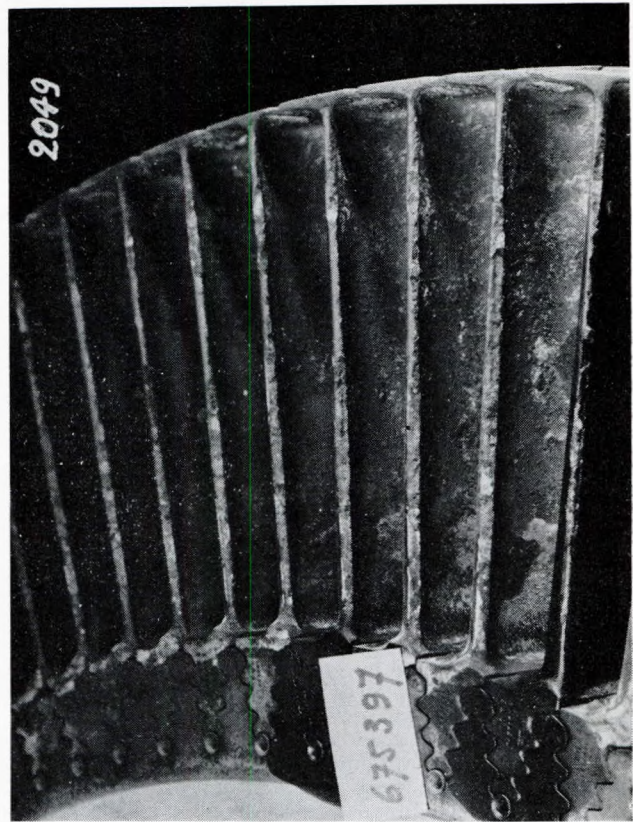
FIG. 16—Typical turbine blade sulphidation
