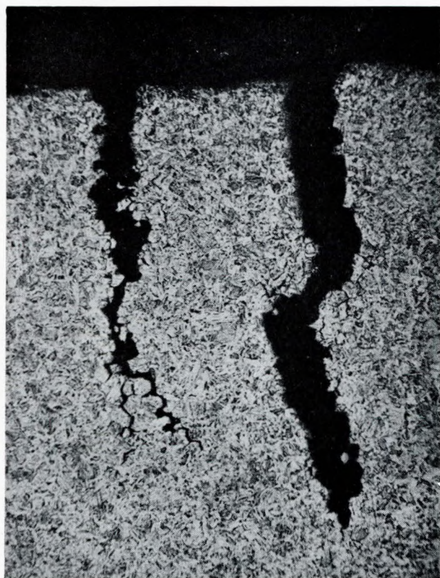
FIG. 4—Typical cracks partially penetrating the failed tube—cracks initiated from the inner wall—magnification \times 50
