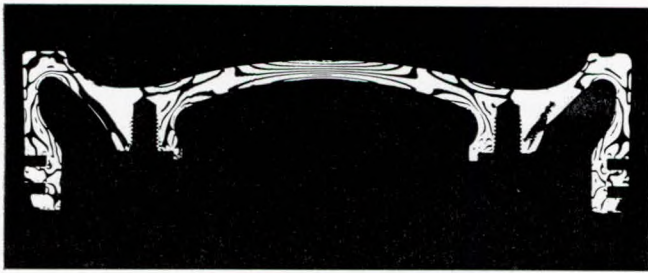
FIG. 13—Photo-elastic test of piston crown— VV52/55 engine
