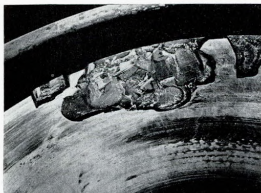
FIG. 9—Distressed area of bearing in Fig. 8
