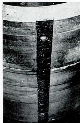
FIG. 11—Dirt and residue in oil slot
