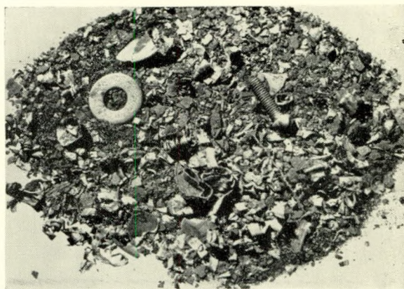
FIG. 14—Debris removed from turbine lubricating oil system
