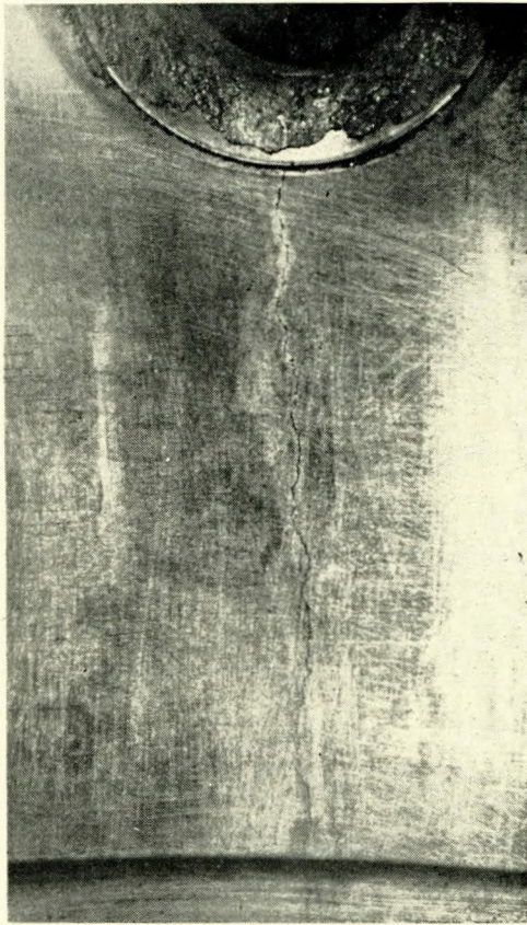
FIG. 2—Cracked cast iron cylinder liner
