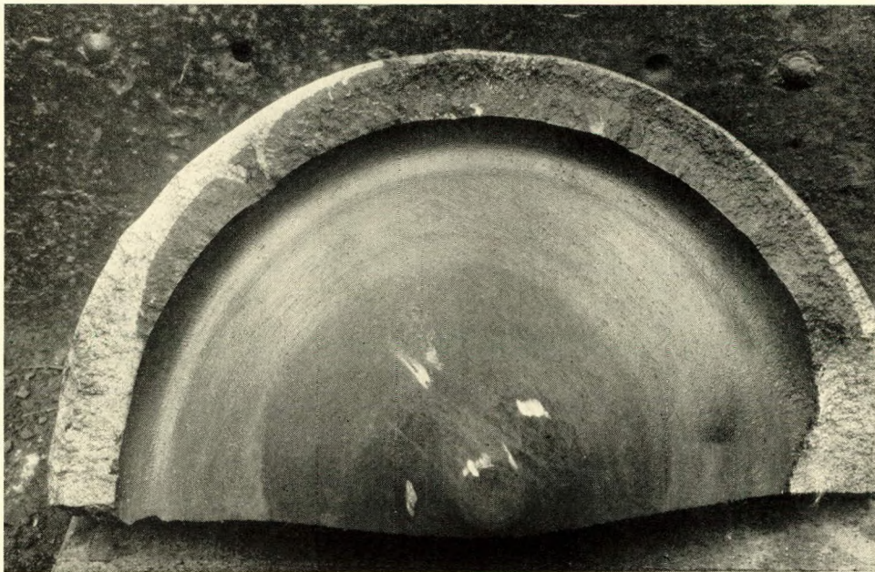
FIG. 7(c)—Crack that was subsequently revealed on breaking up piston
