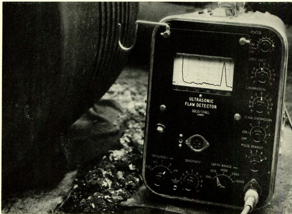
FIG. 7(a)—Flaw detector with quartz crystal probe (transceiver) on sound portion of piston: initial response due to interface echo followed by echo at about 240 mm. deep, i.e. the ring groove
