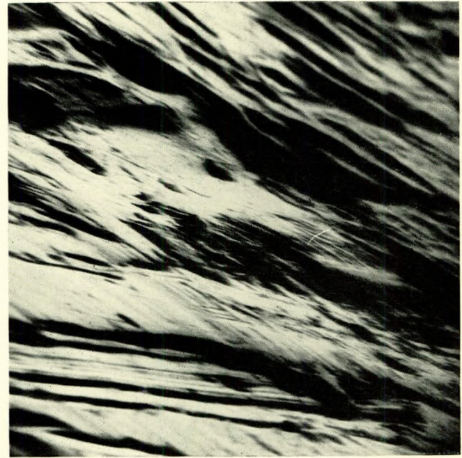
FIG. 5(c)—Reflection electron micrograph: heavily shaved gear
