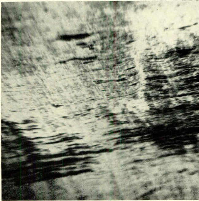
FIG. 5(a)—Reflection electron micrograph: hobbed gear
