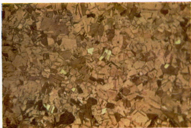
FIG. 4—Photomicrograph showing the structure of alpha brass
