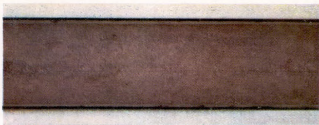
FIG. 1—70/30 brass tube (arsenic-free) attacked by layer type dezincification
