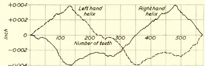
FIG. 10—Typical cumulative pitch errors (main wheel)
