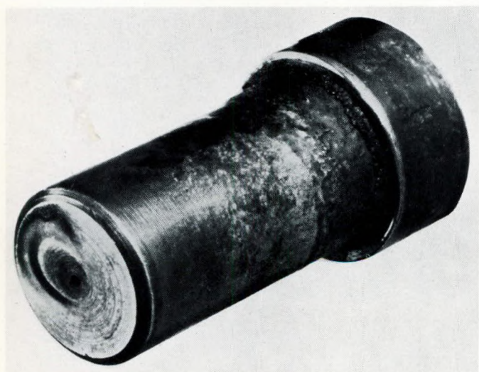
FIG. 14— Nozzle attacked on flat combustion face
