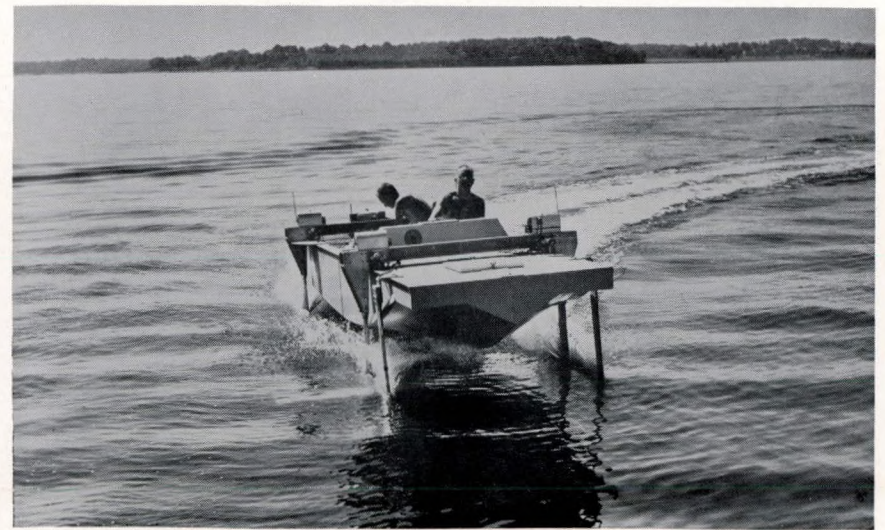
Official photograph U.S. Navy FIG. 10—Automatic incidence control stabilization on a 20-foot United States Navy Test Craft
