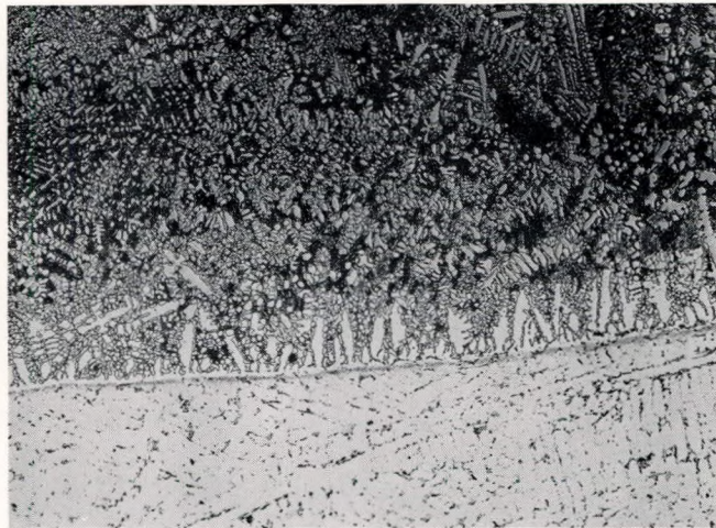
FIG. 16— Fused-on coating of nickel-chromium-boron alloy, showing good adhesion between coating and steel base × 70
