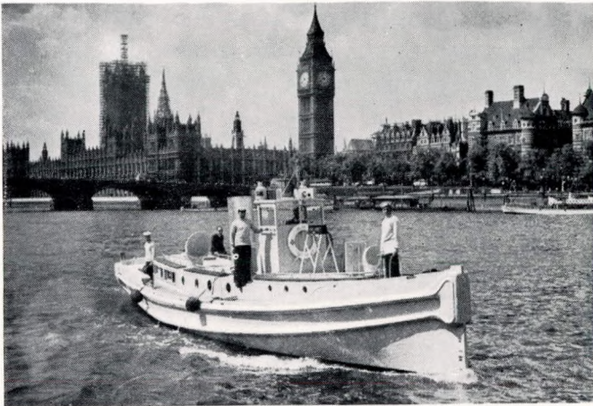
FIG. 26—Gas turbine propelled harbour launch No. 3964 on the Thames By courtesy of the Keystone Press Agency, Ltd.
