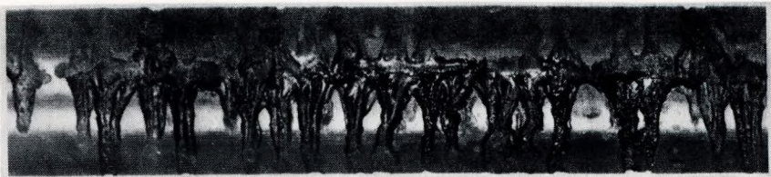
FIG. 19 (top left)—The effect of oil corrosion on the outside of an aluminium brass tube
