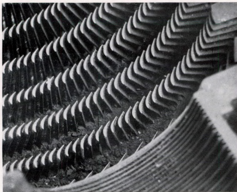
FIG. 6—Photograph showing deposit at bottom of h.p. turbine casing after 636 hours on 1,230 seconds fuel
