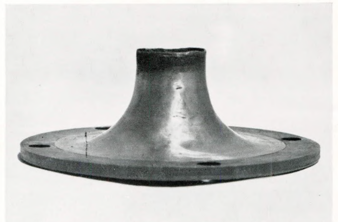
FIG. 14—Modified design of combustion chamber components after 3,529 hours' running on marine Diesel fuel: (a) swirler vanes; (b) lipless shroud
