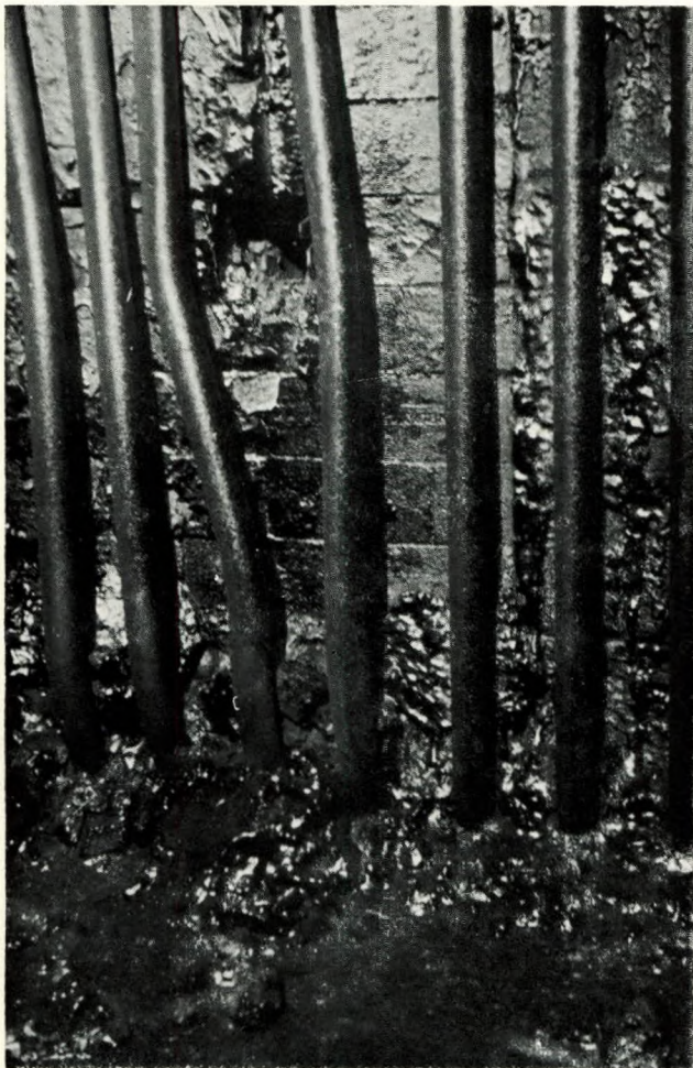
FIG. 27 (above)—Damage to back wall of superheater-side furnace: twin-furnace controlled superheat boiler
