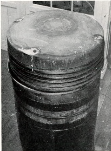
FIG. 18—View on scavenge side of piston after 220 hours' continuous service with 3,000 seconds Redwood I fuel
