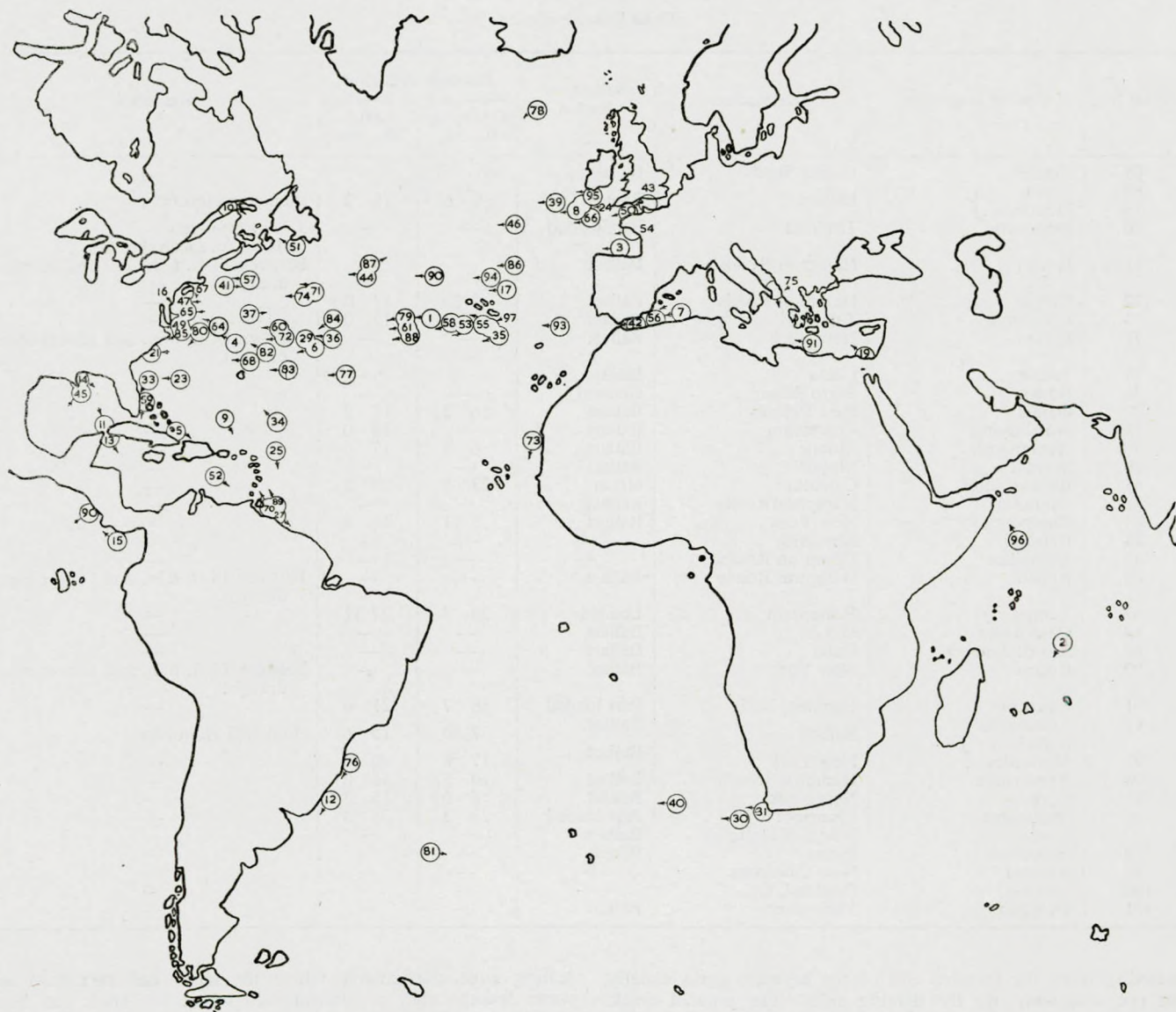
FIG. 4(a)—Geographical location in the Atlantic area of "Liberty" ships at the time of propeller loss
