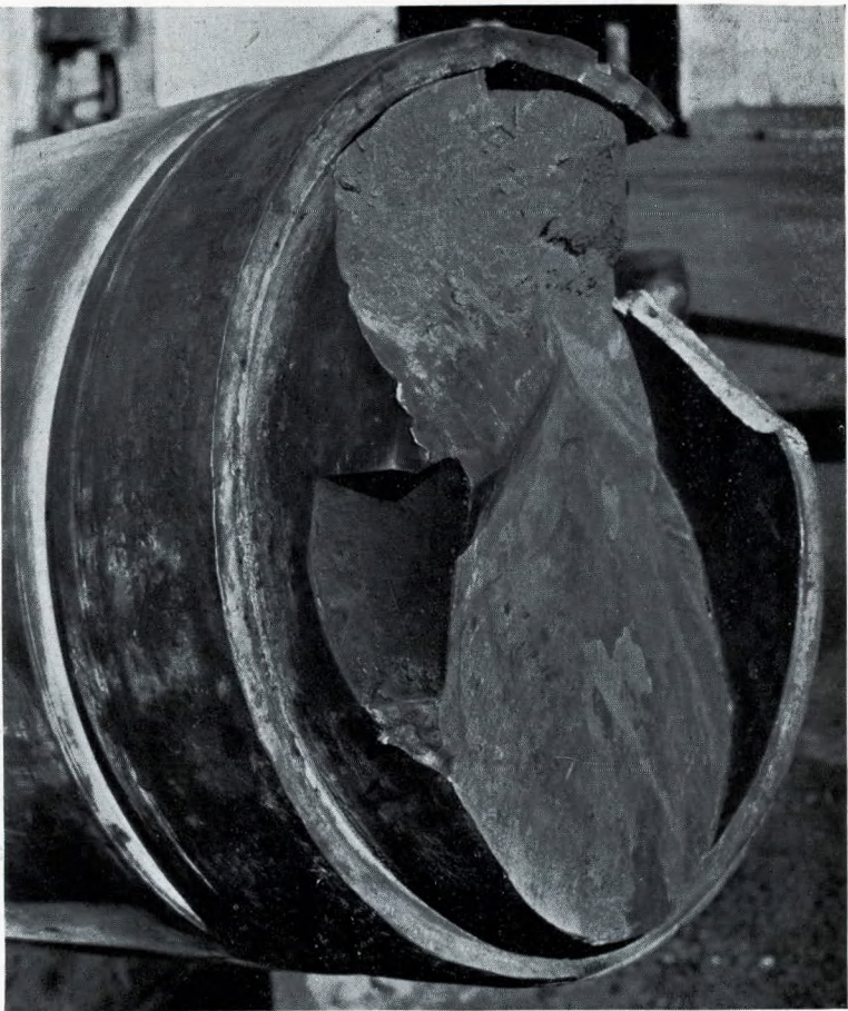
FIG. 10—Fractured “Liberty” screwshaft (see also Fig. 11 for end view)
