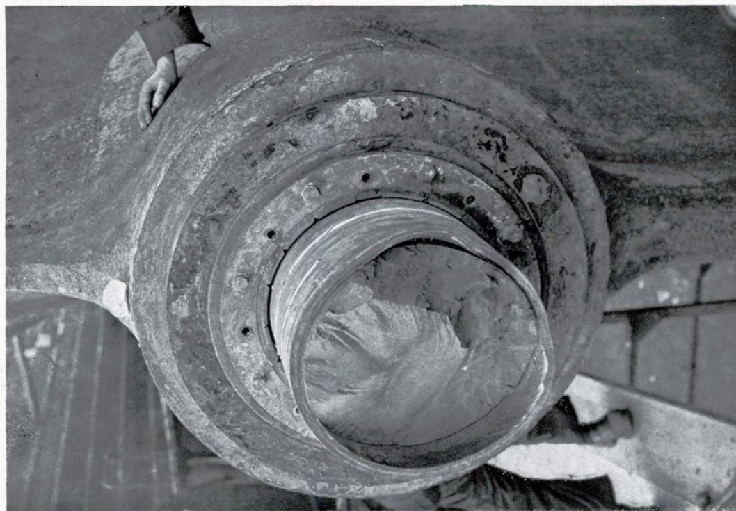
FIG. 7—Typical example of screwshaft failure in “Liberty” type
