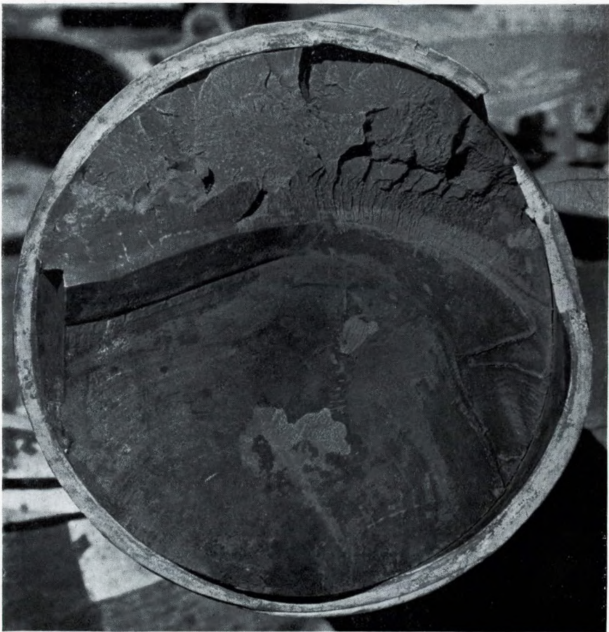
FIG. 11—Fractured “Liberty” screwshaft (see also Fig. 10 for side view)
