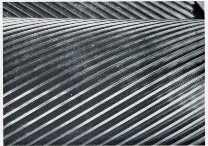
FIG. 9.—Starboard engine pinion at start of experiment (no difference)
