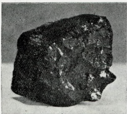
FIG. 11.—A sample of the glass-like slag from the furnace floor of Cruiser "Z".
