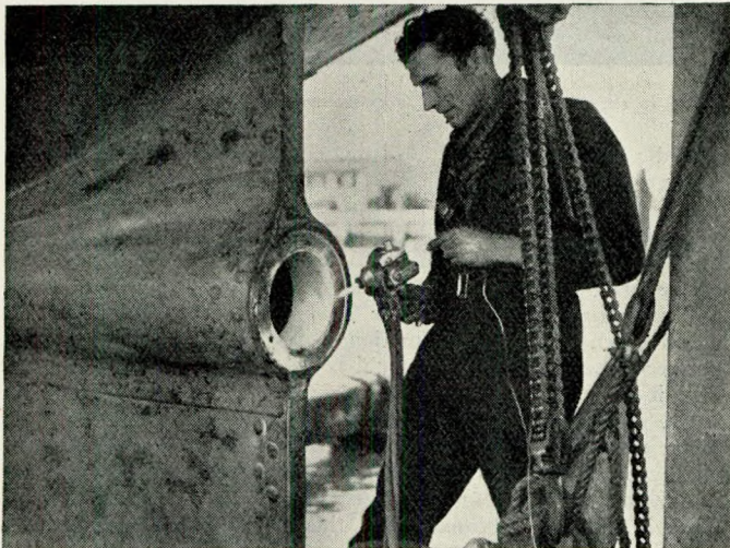
FIG. 20.—Repair of oversize bore in sternpost
