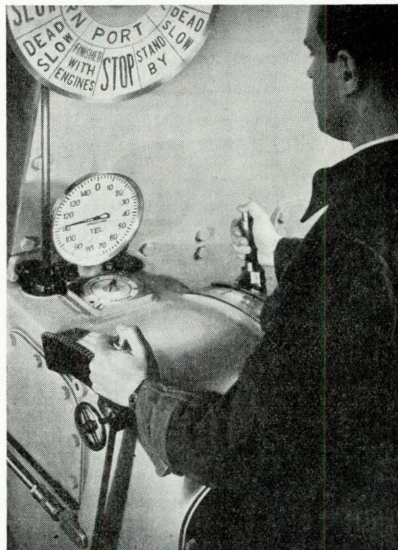
Lever controls of a modern Sulzer engine
