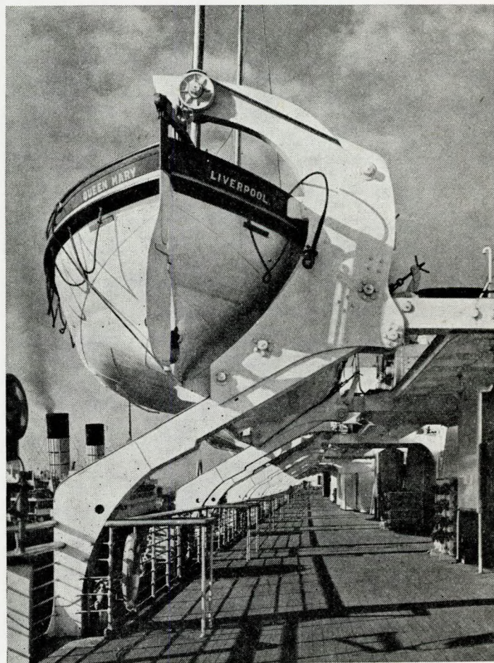
FIG. 7.—The Taylor gravity davit fitted on the q.s.t.s "Queen Mary".
