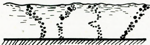
FIG. 5.—Point-evaporation of a boiling liquid.
