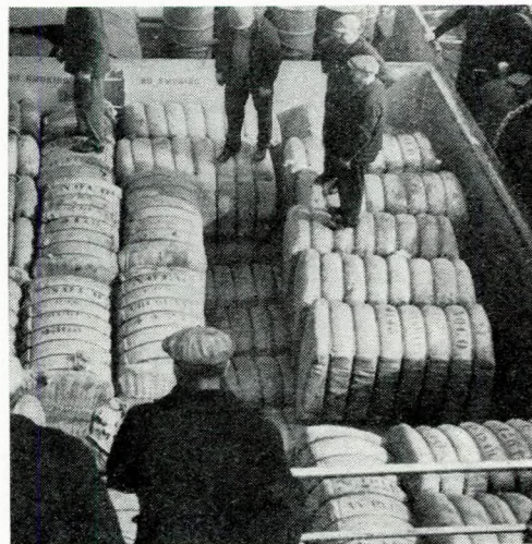
FIG. 13.—Protected No. 2 hatch of s.s. "Mormacmoon" immediately after opening at Boston. No sign of sweat on steel structure and bales in perfect condition.
