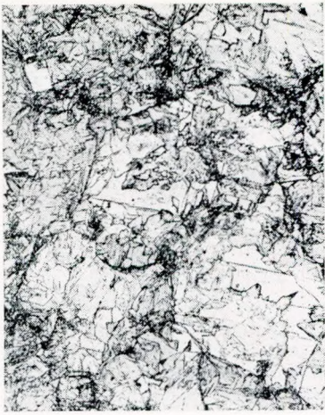
(D) Tempered hardened by heating to 550° C.
