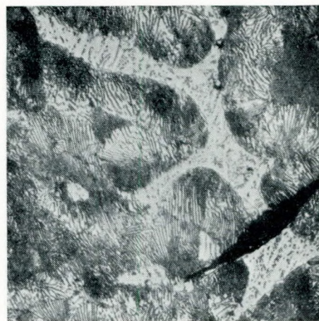
FIG. 11.—All-pearlitic iron containing high phosphorus. Magnification: \times 400 diams.
