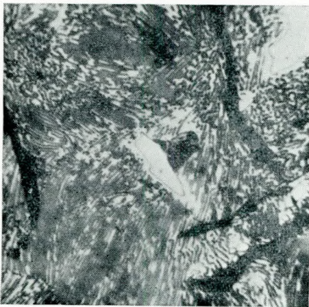
FIG. 15.—Sand-cast 'Loded' iron. All-pearlitic structure (Fig. 7). Magnification: \times 1,500 diams.
