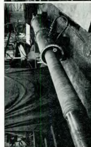
Preparing the shaft for heat-treatment in the shops.
