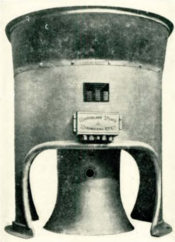
FIG. 5.—Fan for vertical air flow.
