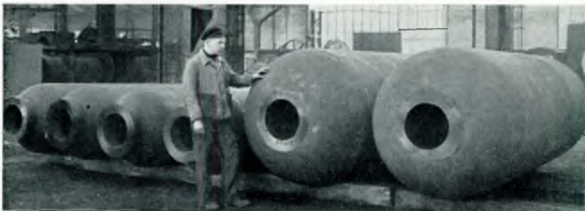
FIG. 27.—Forged welded steam drums and radial-rolled water drums.
