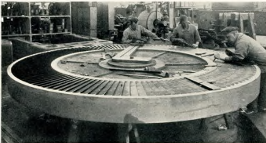
FIG. 20.—Checking the guide passages in a nozzle ring.
