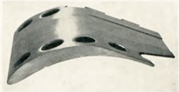
FIG. 21.—Thick blade for cast-in type nozzle.
