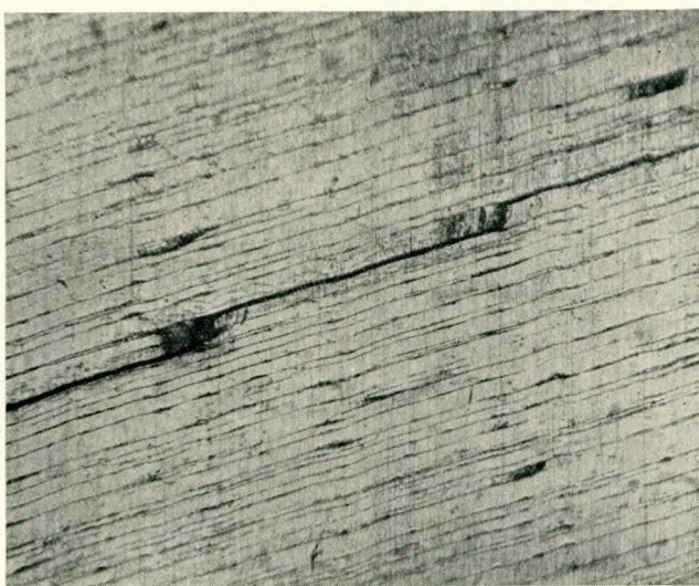
FIG. 15.—Slip bands and fatigue cracks in a single crystal of aluminium.
