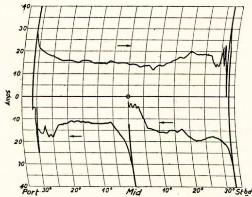
FIG. 2.—Current consumption of steering gear during one manœuvre.
