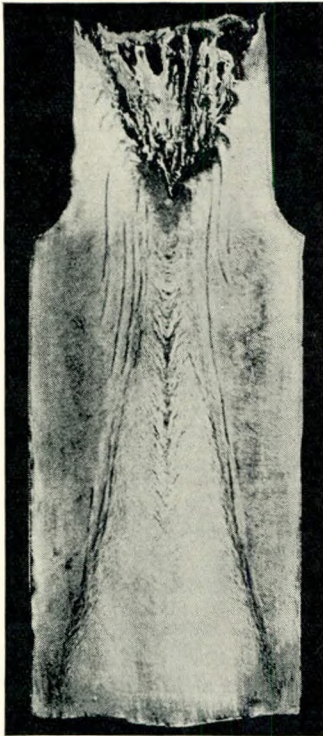
FIG. 1.—Longitudinal section through large forging ingot showing cavity in head and segregation. (1st Report on the Heterogeneity of Steel Ingots.—Iron and Steel Institute).
