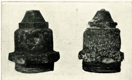
Fig. 8.—Corroded Fusible Plugs from Marine Boilers.
