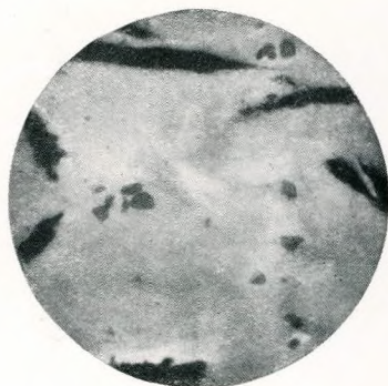
Fig. 16. Sulphide "Globules" in Cast Iron. Magnified 100 diameters.
