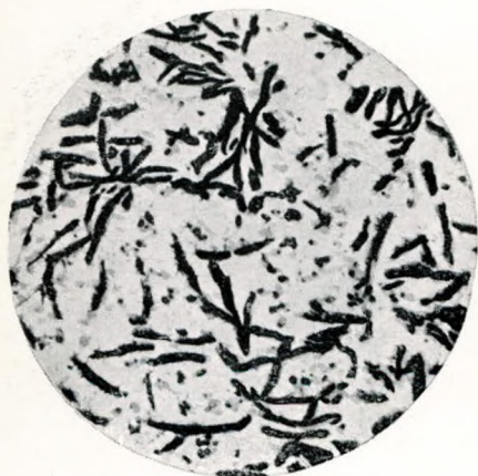
Fig. 9. Testbar cut out of Liner. Showing Graphite. Magnified 25 diameters.
