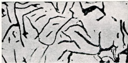
Fig. 19. Graphite in same Cast Iron after growth. Magnified 100 diameters.
