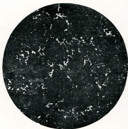
Fig. 14. Good Phosphide Network in Cast Iron. Magnified 25 diameters.
