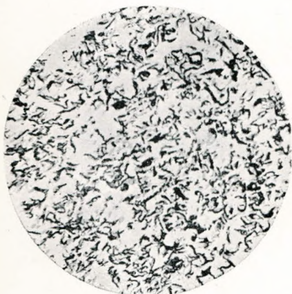
Fig. 7. Testbar cast on Liner. Showing Graphite. Magnified 25 diameters.
