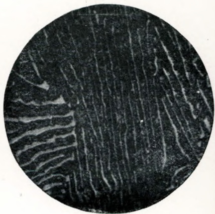
Fig. 10. Testbar cut out of Liner. Showing Pearlite. Magnified 1,100 diameters
