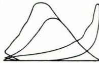
FIG. 8.—Exhaust Temp. 460° C. Scav. Pressure. 3.5 m. of water. P_e = 7.55 kg. per sq. cm. P. \text{ max.} = 51 kg. per sq. cm. Comp. Press. = 37.5 kg. per sq. cm.
