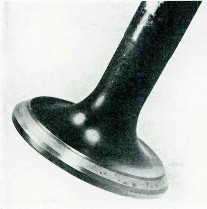
FIG. 2.—Exhaust valve after using light distillate fuel.
