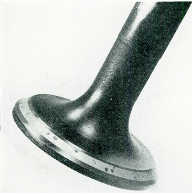
FIG. 3.—Exhaust valve after using Stream-Line treated Diesel fuel.
