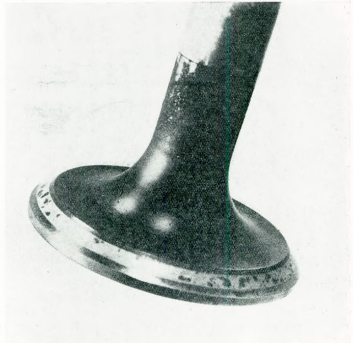
FIG. 4.—Exhaust valve after using the same fuel as for Fig. 3 but untreated.
