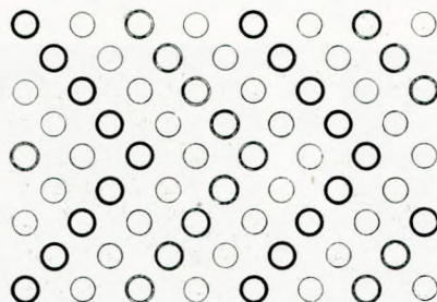
FIG. 2 (Upper).—Showing the disposition of the long and short tubes. FIG. 3.—Arrangement of tubes for turbulence.
