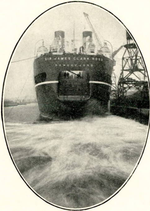
Basin trials with the starboard engine.
