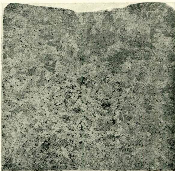
Fig. 17.—Vertical section of Y-alloy ingot cast in open sand mould without feeding. Full size.
