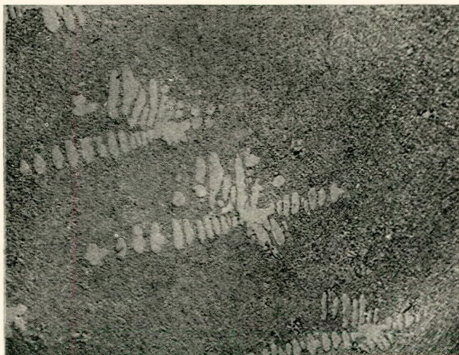
Fig. 13.—Silicon-aluminium alloy. Modified structure X150.
