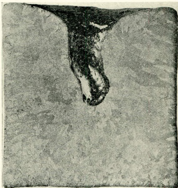
Fig. 15.—Vertical section of aluminium ingot cast in open sand mould without feeding. Full size.
