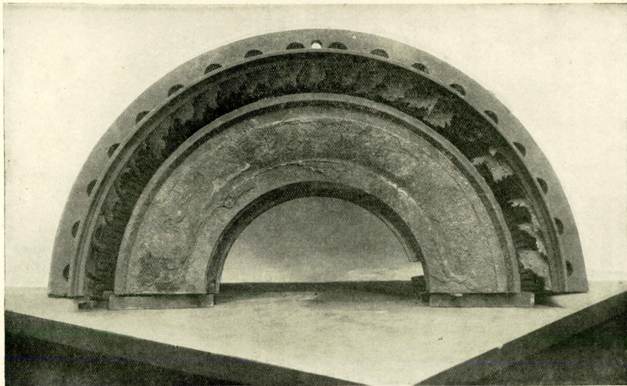
This illustration is reproduced from a photograph forwarded by Capt. P. T. Brown (Member) to show the severe corrosion on a turbine
