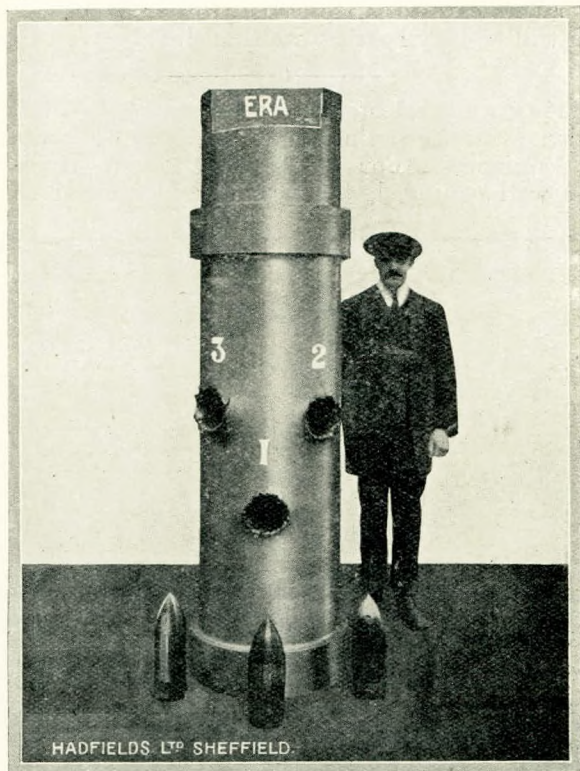
Portion of Marine Shaft of Hadfield's Special Quality "Era" Steel after attack by 20½ c.m. armour-piercing projectiles.
