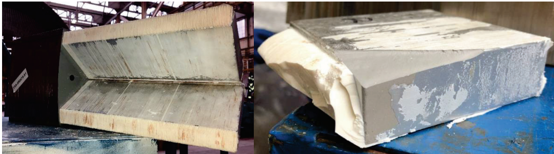
Figure 10: Post test strip-down of test sample: no sign of damage was found on the magnets and rotor components.
