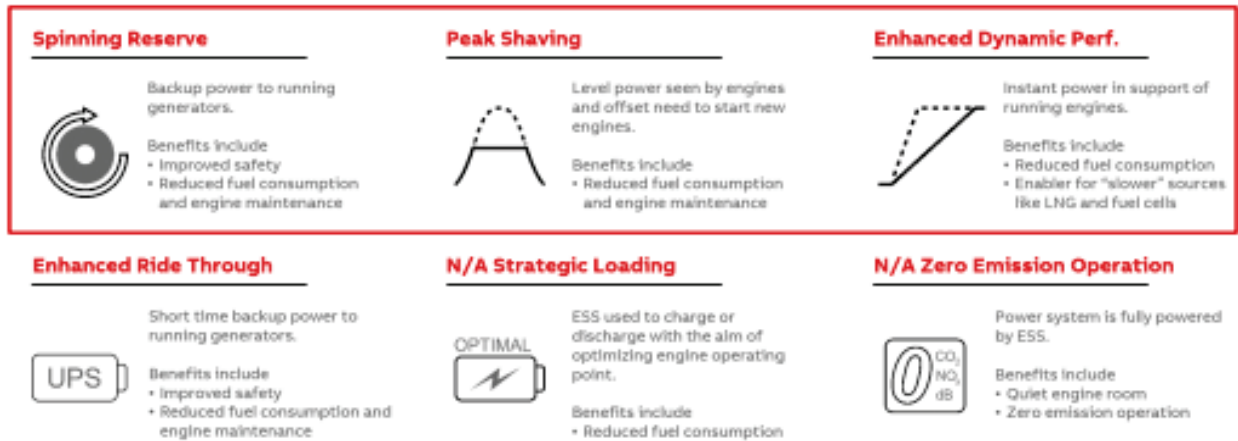
Figure 1 - shows an overview of the BESS functions in a DC power system, with the focused functions discussed above highlighted
