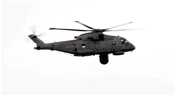
Figure 1 - Merlin Crowsnest with Radar Dome Lowered (Royal Navy, 2021)
