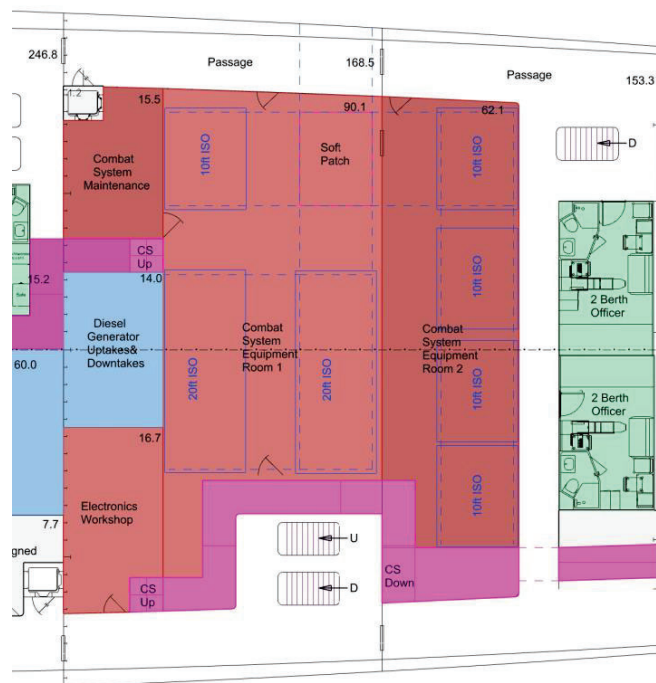
Figure 3: Combat system equipment room modular installation example.
