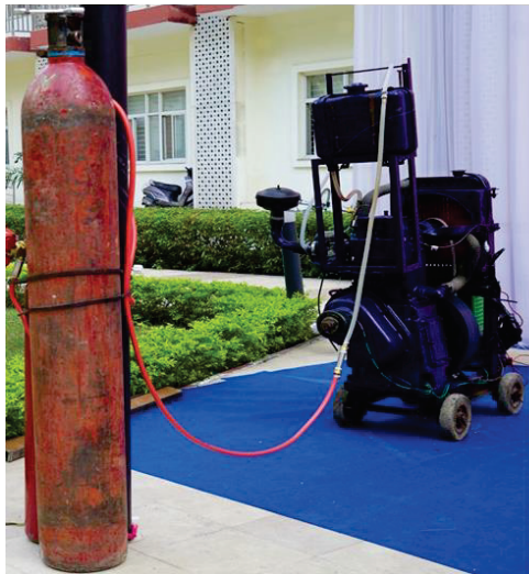
Figure 13: The detailed engine schematic alongside a demonstration of the hydrogen-powered diesel engine
