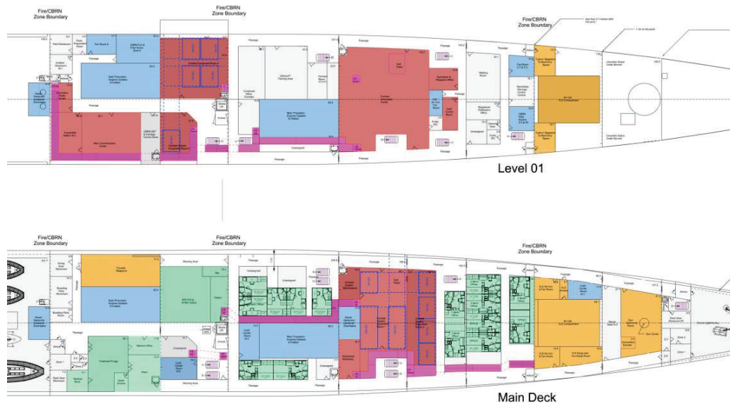
Figure 2: Indicative implementation of combat system enclaves (red) linked by galleries (pink).
