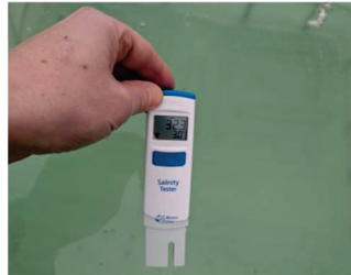
Figure 12 – Output of qualitative drench test in saltwater
