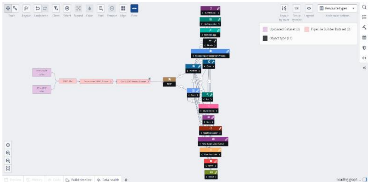
Figure 8: Foundry Pipeline Builder enables the concept sketch to be transformed into an automated data pipeline, where laboratory results of oil analysis are turned into usable Objects in the digital mother. It uses relational links to Asset and Platform to facilitate trend analysis with a variety of other objects.
