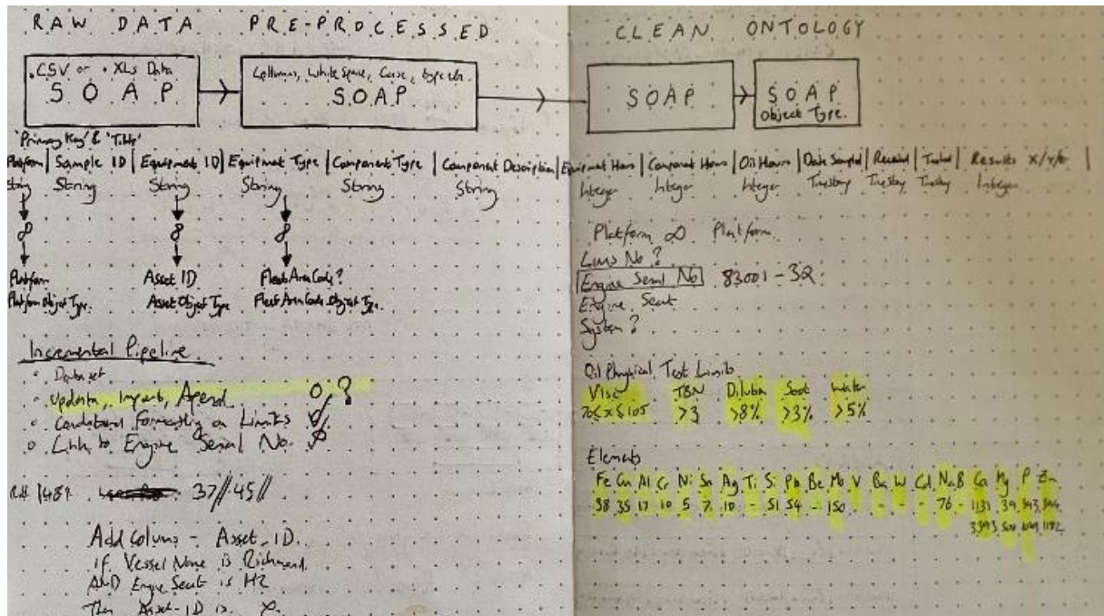
Figure 7: Concept sketch of the data-pipeline used to ingest Spectrometric Oil Analysis Programme (SOAP) data with steps for pre-processing, cleaning, and the assignment of a Foreign Key to enable relational links into other datasets such as Assets and Platforms.
