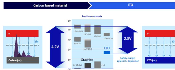
Figure 8 – How LTO compares with Graphite/Carbon Anode
