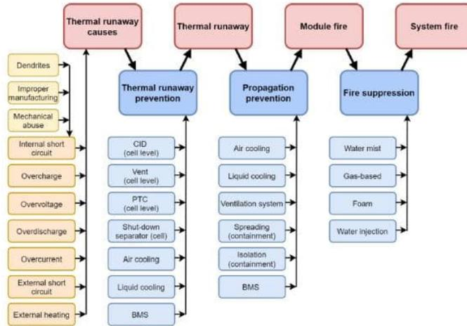
Figure 7– Causes and prevention methods of TR [4]
