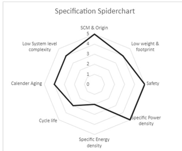
Figure 5 – Main criteria and importance (1-5) for BESS design
