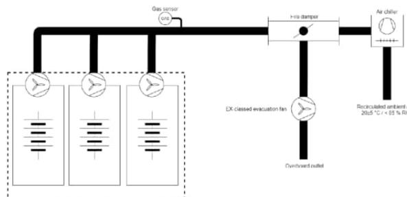
Figure 11 – Notional picture on aircooled LTO Strings with combined gasevacuation and cooling duct. Note that the separate Battery Room ventilation is not indicated in figure.
