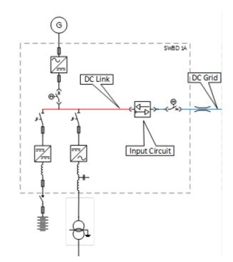
Figure 3 – Notional SLD detail for a combatant damage zone BESS integration. Note complete e.g. four split configurations and SLD can be commercially sensitive and thus is not presented
