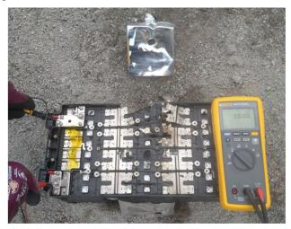
Figure 9 - Overcharge/Overdischarge/Overcurrent/Overvoltage/external short circuit
