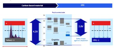
Figure 8 - How LTO compares with Graphite/Carbon Anode
