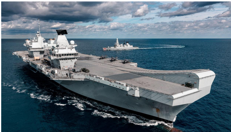
Figure 5 - HMS Queen Elizabeth - A 110MW Power System with a Large Flight Deck and Hangar (Credit: crown copyright 2020)
