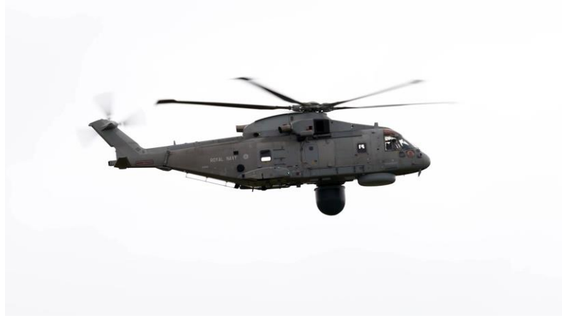
Figure 1 - Merlin Crowsnest with Radar Dome Lowered (Royal Navy, 2021)
