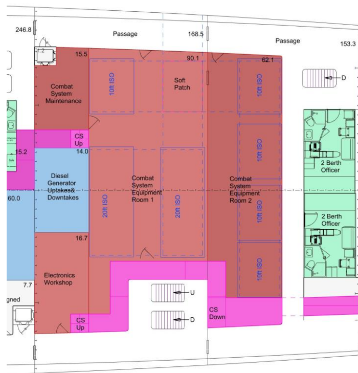
Figure 3: Combat system equipment room modular installation example.
